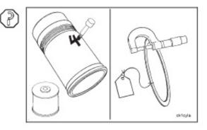
Caution: The liner puller must be installed and used as described to avoid damage to the cylinder block.
